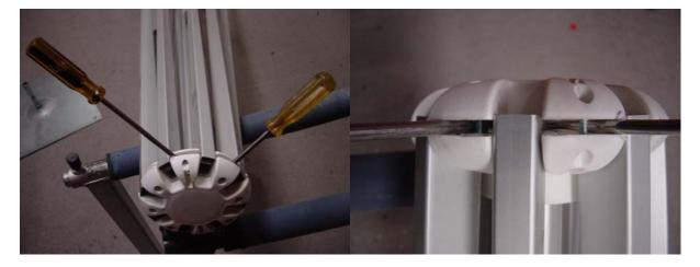
Remove the arm being careful not to loose the pin that holds the arm in place inside the disc. Replace with a new arm and reverse the procedure to complete the repair.
