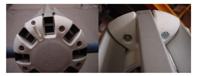
Insert the flat head screwdrivers between the two plastic discs either side of the broken arm and gently pry apart.
